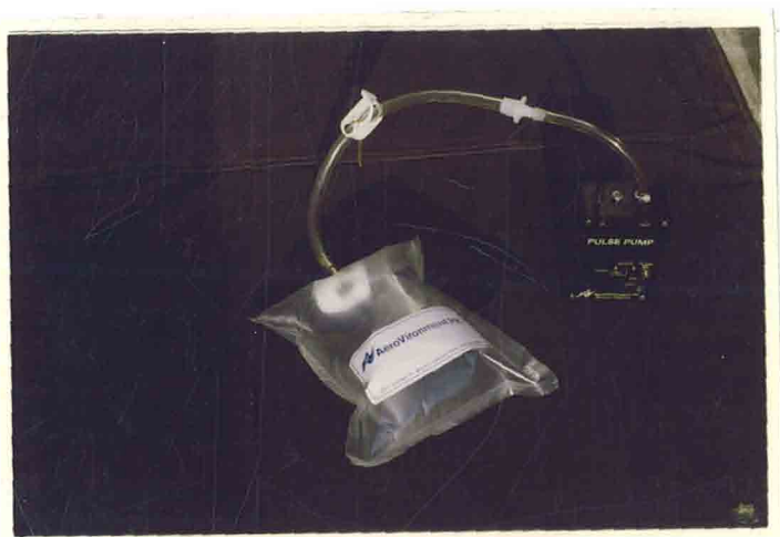
Plate 11 Methane and Carbon di oxide collection chambers used in this investigation.
