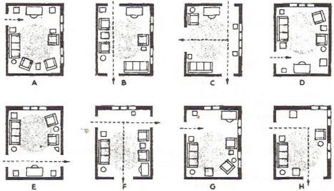
Fig 4.1.44 - living rooms considered from the point of view of possible furniture groupings and interference by necessary circulation. Circles indicate conversational groups dotted lines show circulation.
