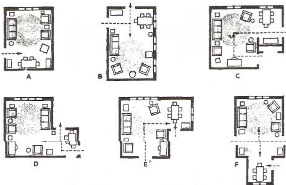
Fig 4.1.45 - a relationship similar to fig complicated by adding constantly used dining space
