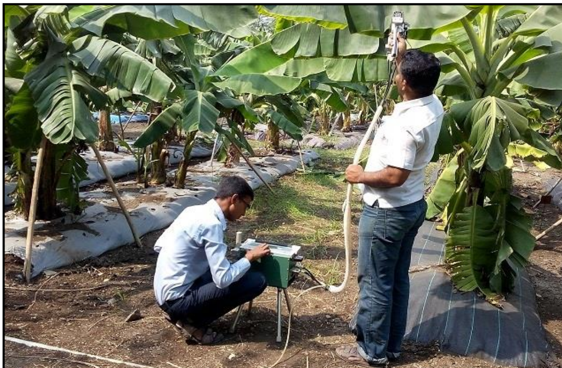
Plate 3.3. Measurement of photosynthesis rate of banana crop
