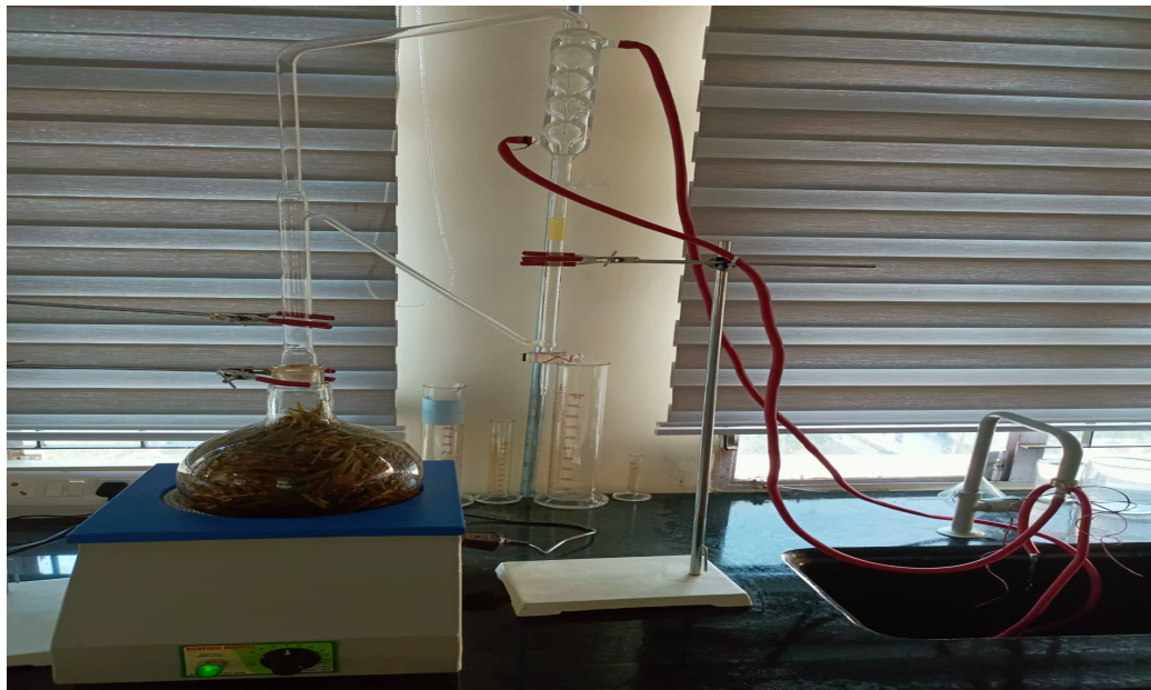
Plate 4: Extraction of lemongrass essential oil by using Clevenger-type apparatus
