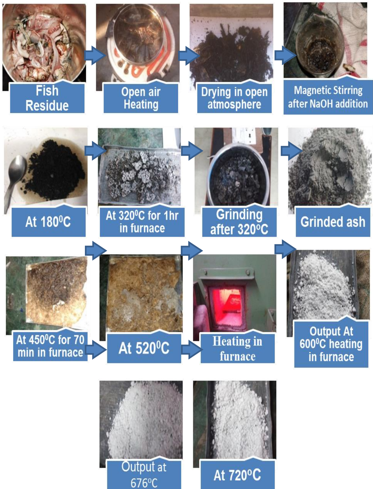
Figure 3.6: Step by step processing performed during extraction of fish residue powder
