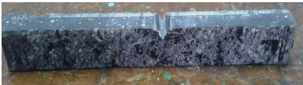
Figure 3.15 (b): Actual specimen for impact testing
