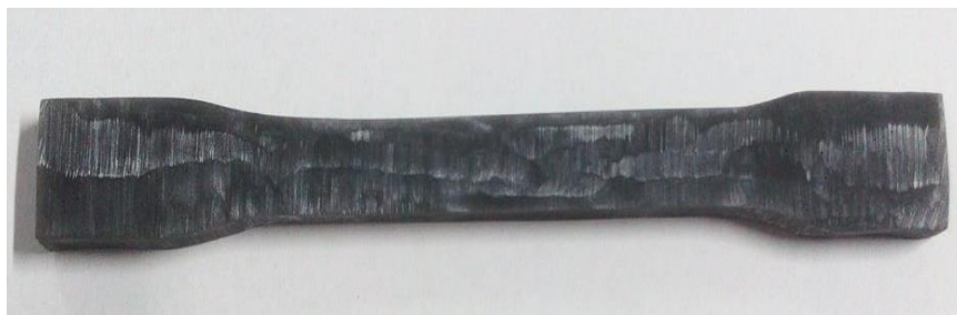
Figure 3.13 (d): Actual test specimen for tensile testing
