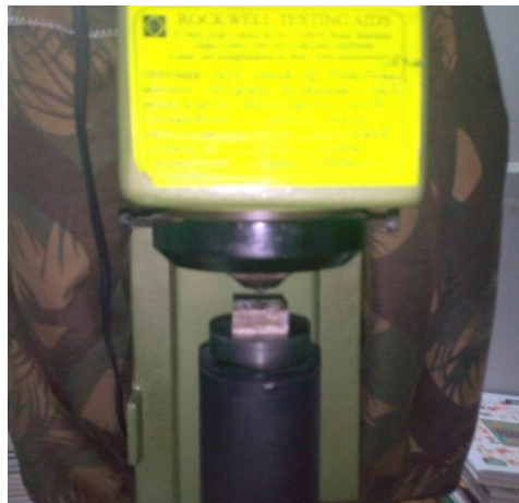
Figure 3.16: Placing of finished specimen for hardness testing
