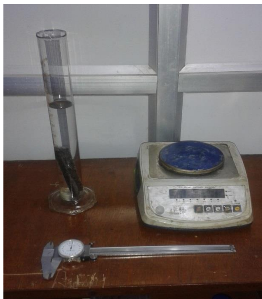
Figure 3.19: Experimental setup for water absorption and thickness swelling test
