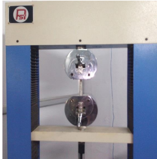
Figure 3.13 (b): Clamping of tensile test specimen on UTM
