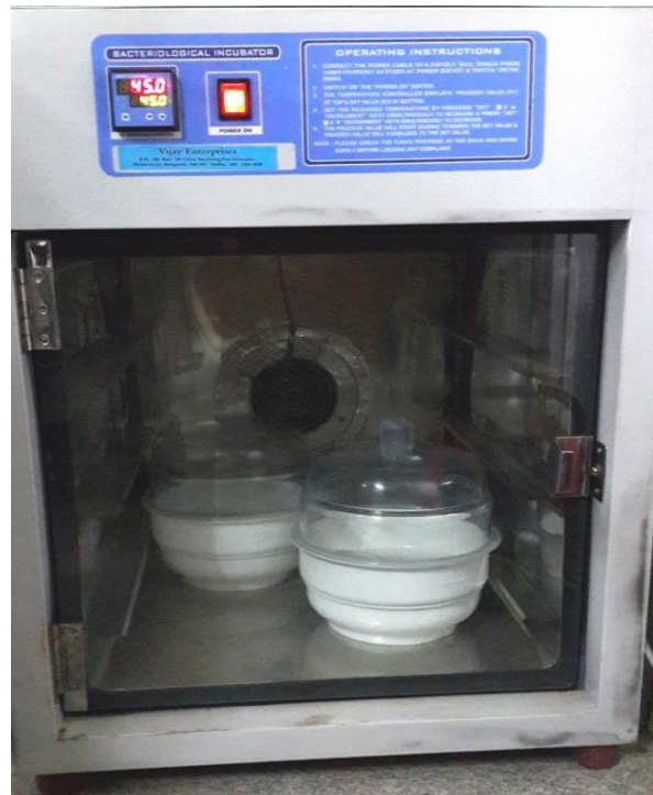
Plate 1: Experimental set up for accelerated ageing
