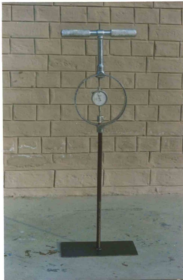
Plate 3.7 Penetrometer device to measure sinkage resistance of puddled soil
