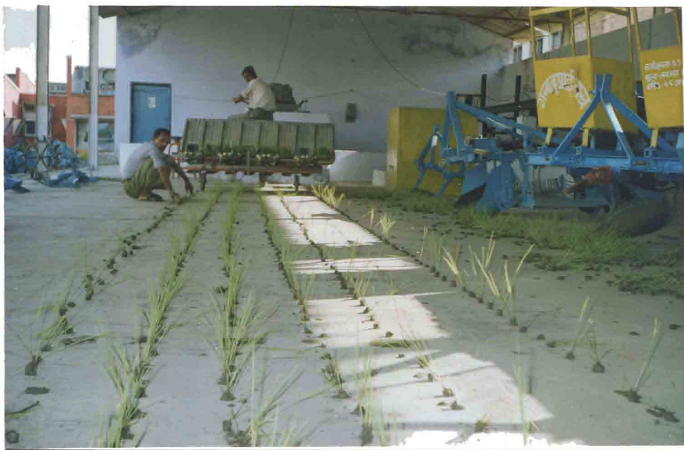
Plate 3.5 Laboratory study of seedling parameters affecting transplanter performance
