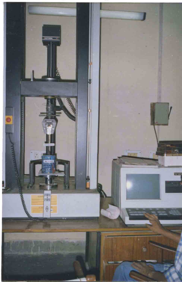
Plate 3.6 Measurement of seedling withdrawal force by using Instron Universal Testing Machine
