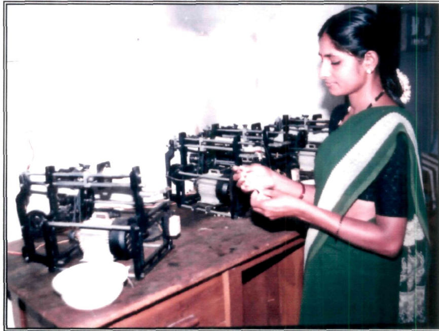
Plate 5: Spinning Ahimsa silk on motorized machine
