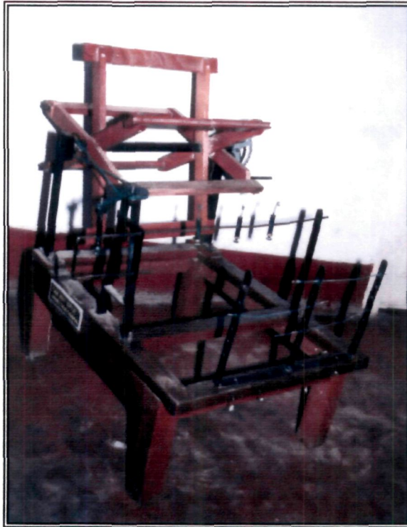
Plate 7: CSTRI rewinding machine
