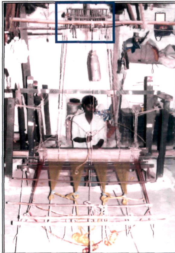
Plate 30: Fly shuttle pitloom with dobby attachment
