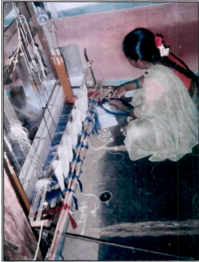
Plate 26: Twisting and joining (piece work)
