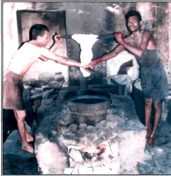
Plate 10: Degumming of Ahimsa silk
