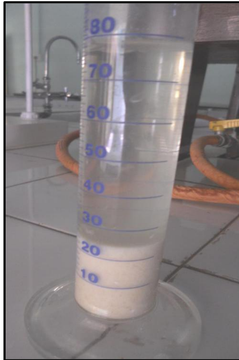
Plate 3.8: Sedimentation value measurement
