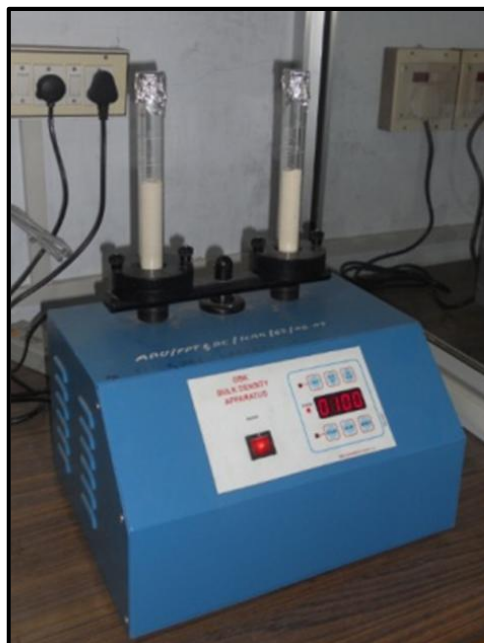
Plate 3.9: Bulk density apparatus
