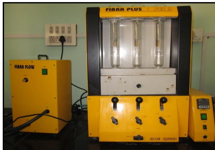
Plate 3.7: Fibra plus equipment used for measuring the fibre content
