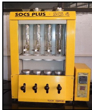
Plate 3.6: SOCS plus equipment used for measuring the fat content
