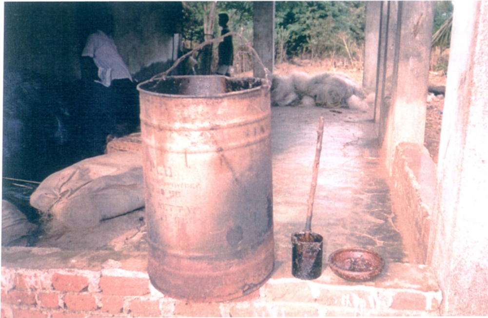
Figure 5 Iron barrel used for preparing the chandrus + oil solution; a small vessel with handle to take it out and earthen dish used to apply the solution to the crafts in Mumbai district
