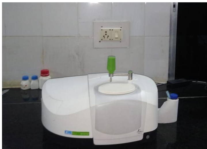
Fig: 2.5 Nicolet 1S5 Mid Infrared FTIR spectrophotometer used for analyzing the films
