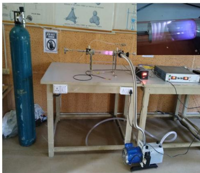
Fig: 2.3 Experimental set up for plasma treatment.
