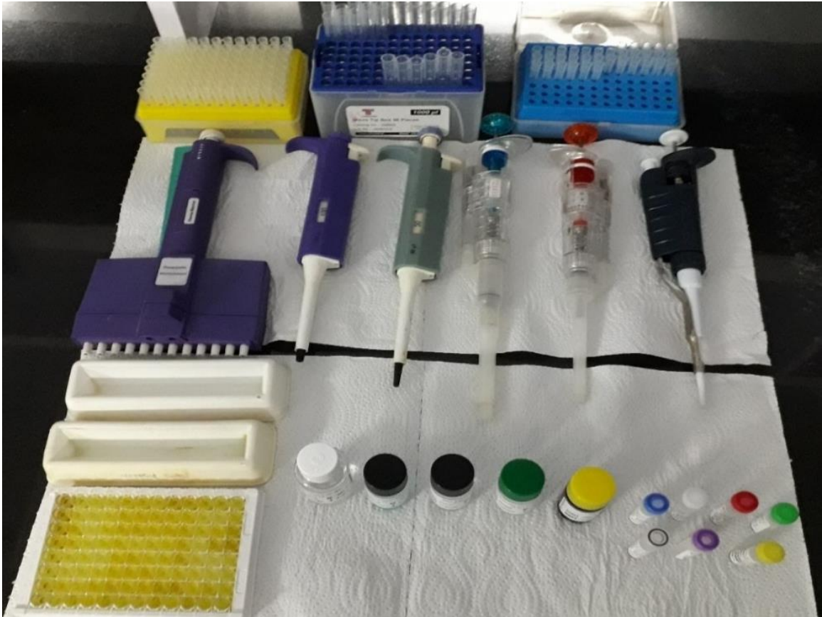
Plate 2. From top to bottom: Microtips, Micropipettes, Solution holding boats, ELISA plate and ELISA reagents for ELISA
