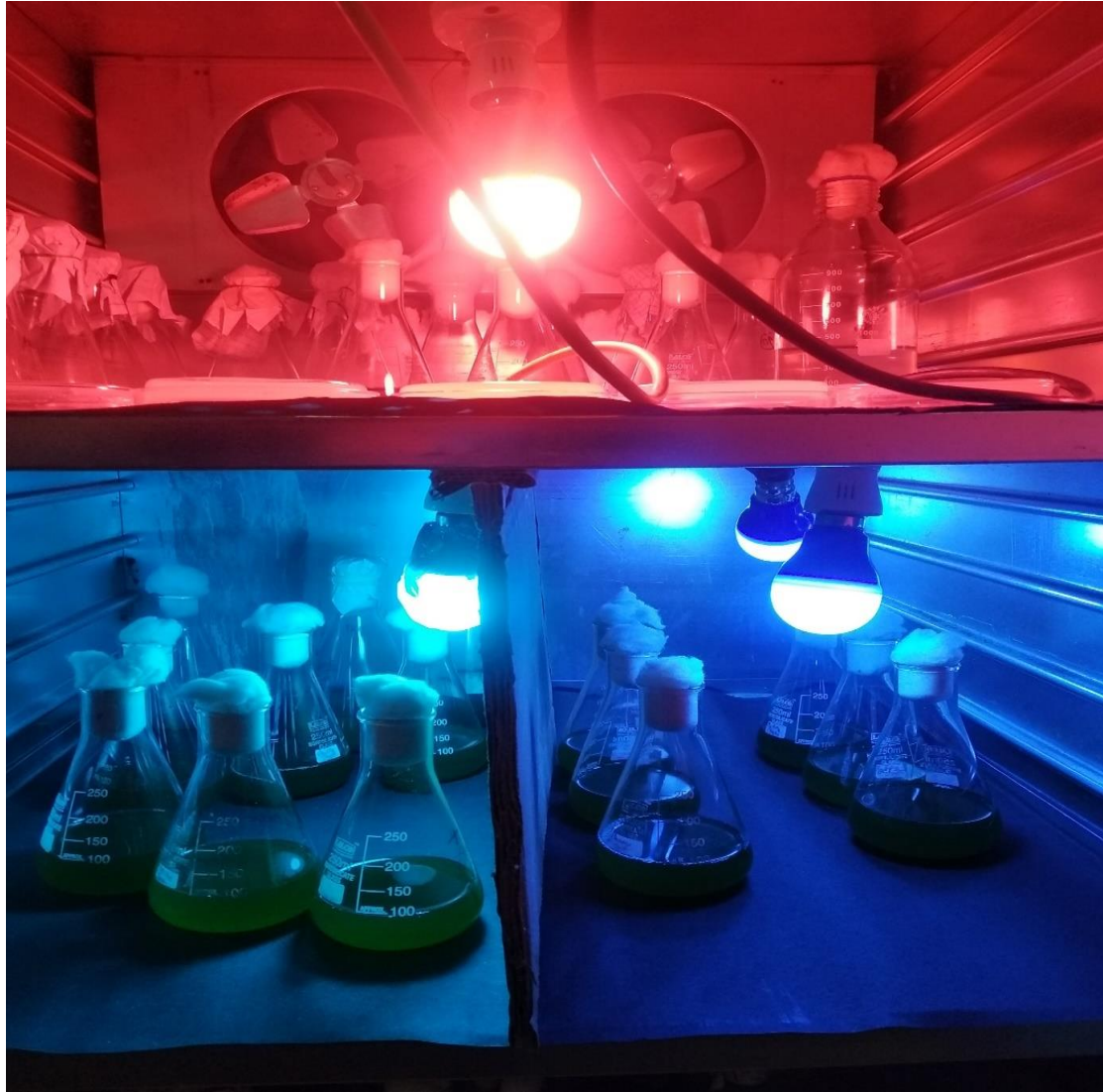
Plate 8. Setup for observing the effect of different light-shifting strategies on the accumulation of astaxanthin
