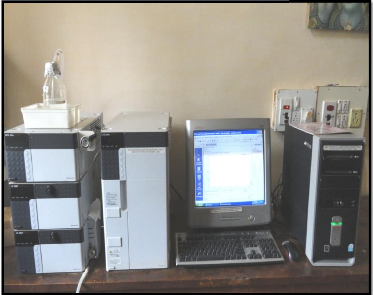
Plate 5 : High Performance Liquid Chromatography which is used to determine phorbol esters
