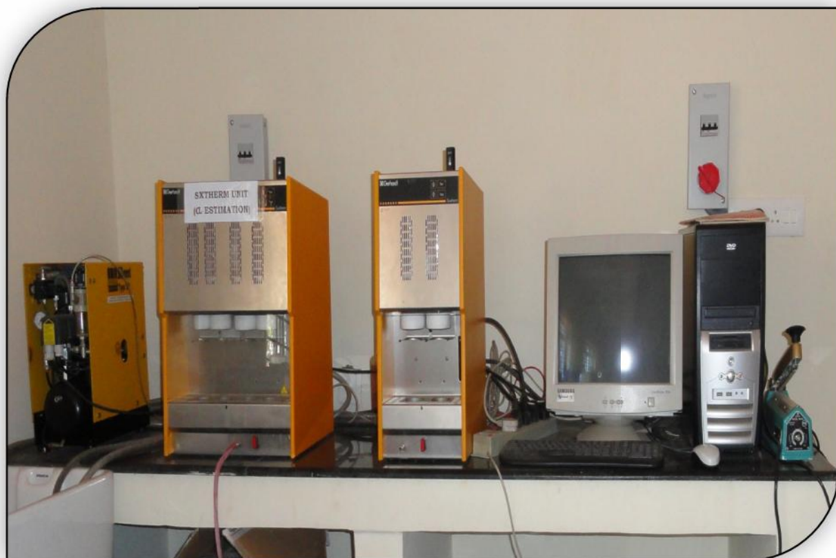
Plate 4 : Soxtherm apparatus used for extraction of oil
