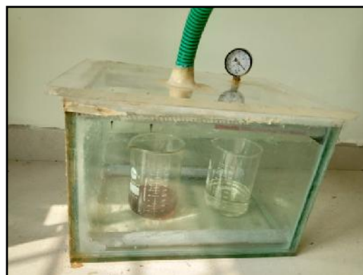
Fig I. Vacuum chamber used for resin impregnation into helminths
