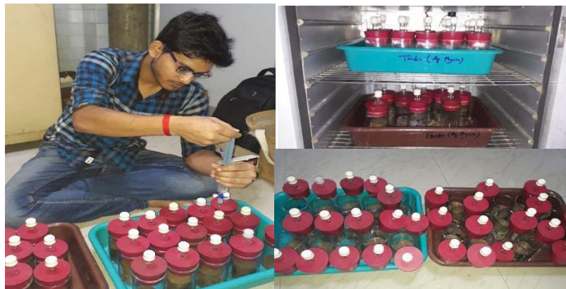
Figure 3.6: CO 2 sampling for monitoring carbon mineralization
