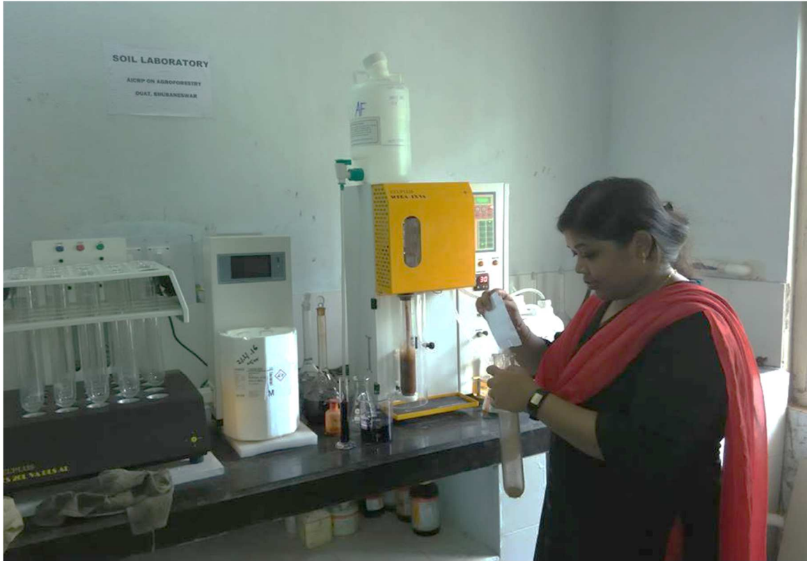
Fig. 3.4 Analysis of soil samples using KEL PLUS Nitrogen analyser
