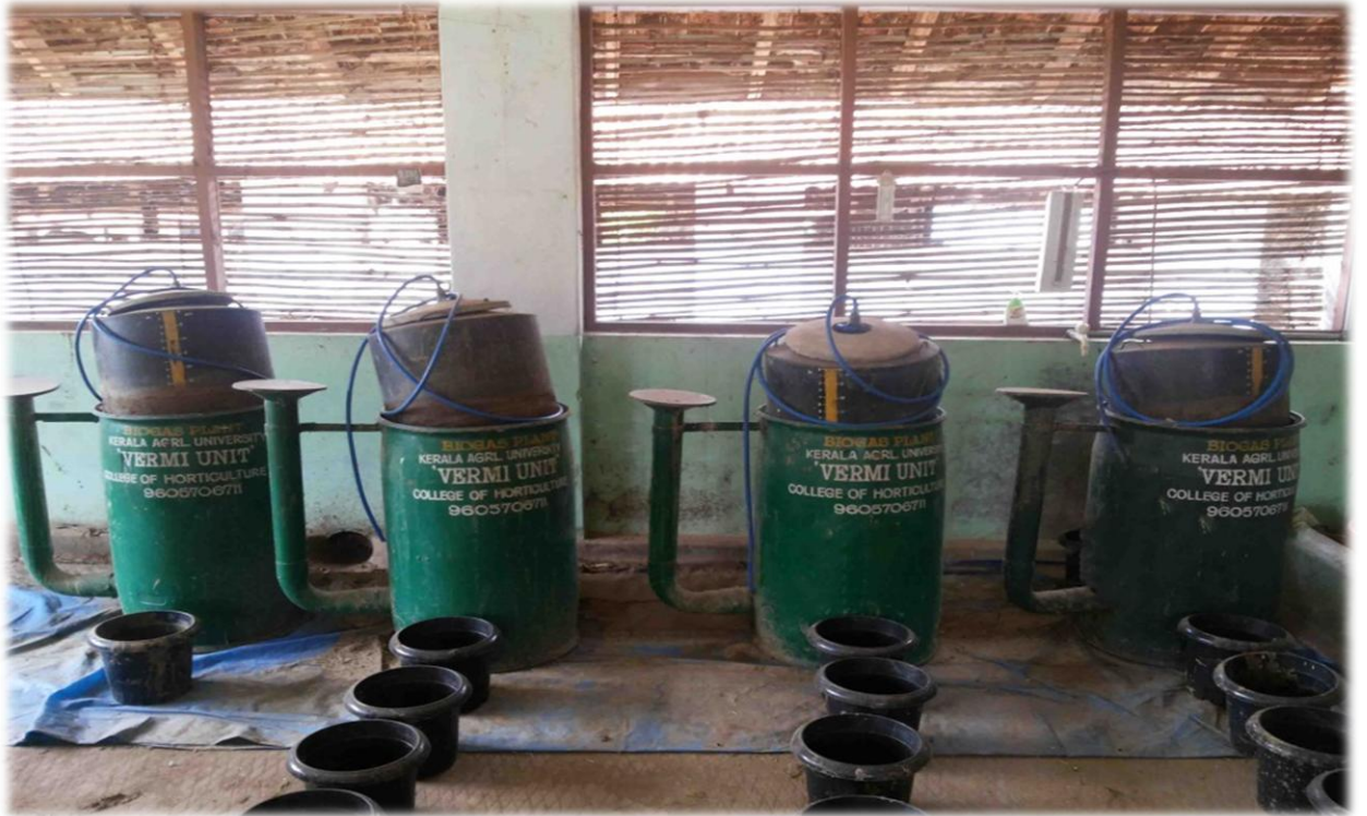
Portable Floating drum type Biogas plant of 0.5 m 3 capacity
