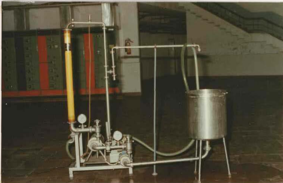
PHOTO PLATE 2 : ULTRAFILTRATION PLANT
