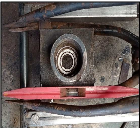
(c) Bearing housing with mounting
