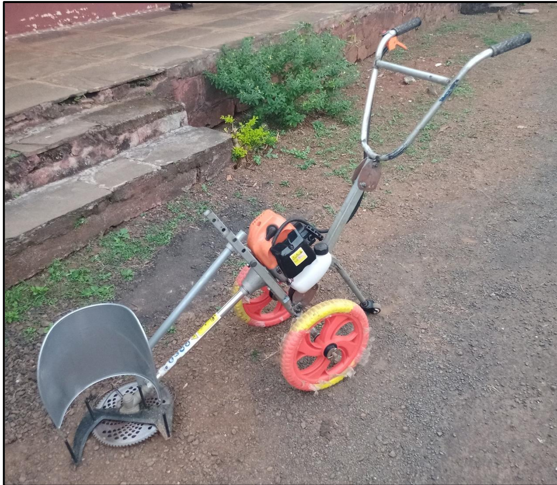
Plate 3.11. Developed prototype of grass cutter cum paddy harvester
