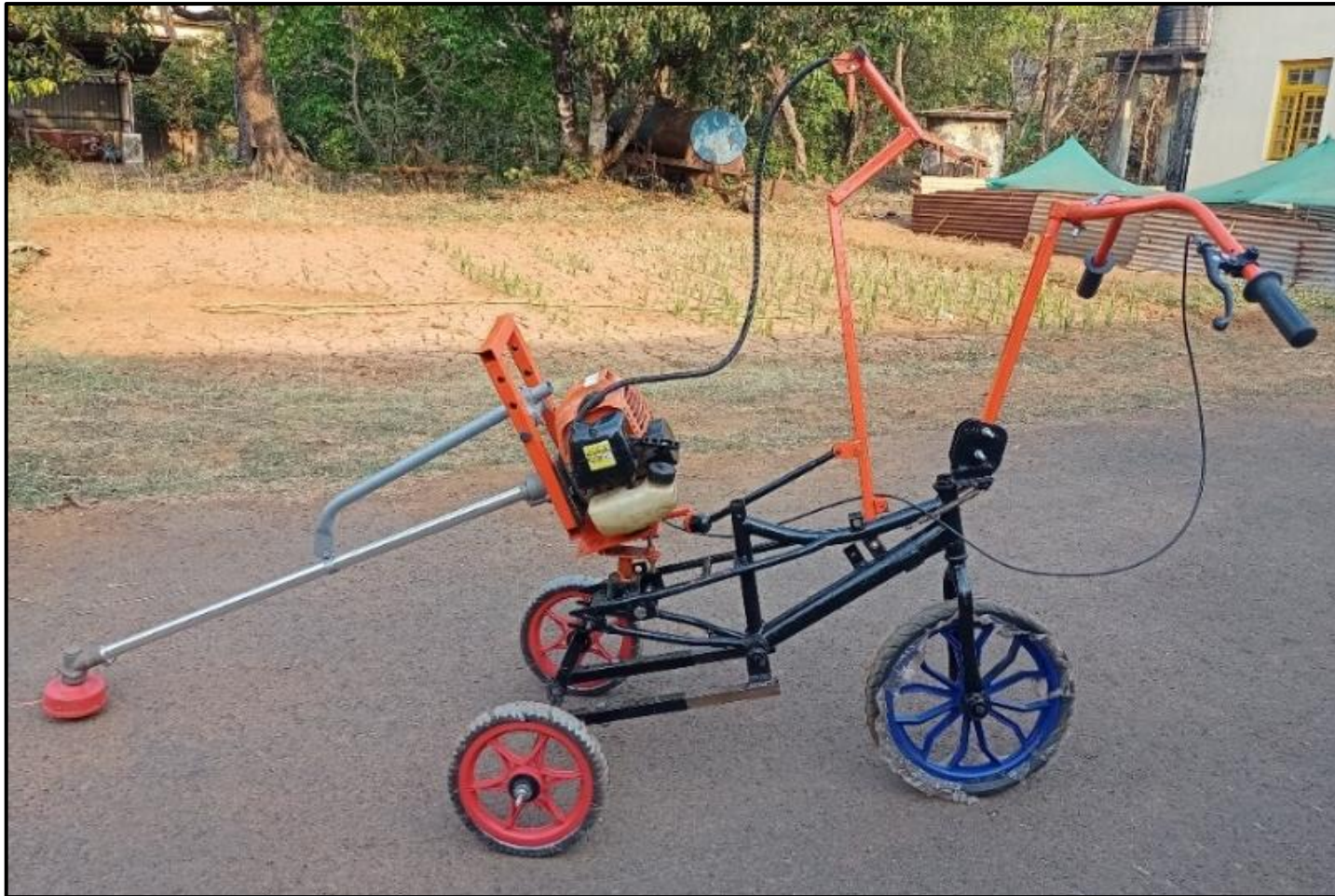
Plate 3.15 Developed second prototype of grass cutter cum paddy harvester
