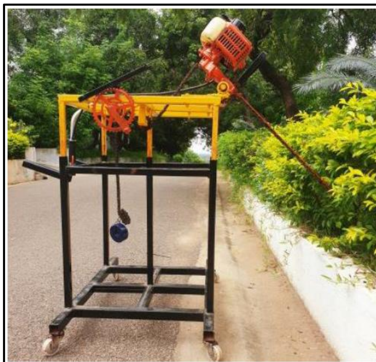
(b) Hedge trimming machine with angular adjustment
