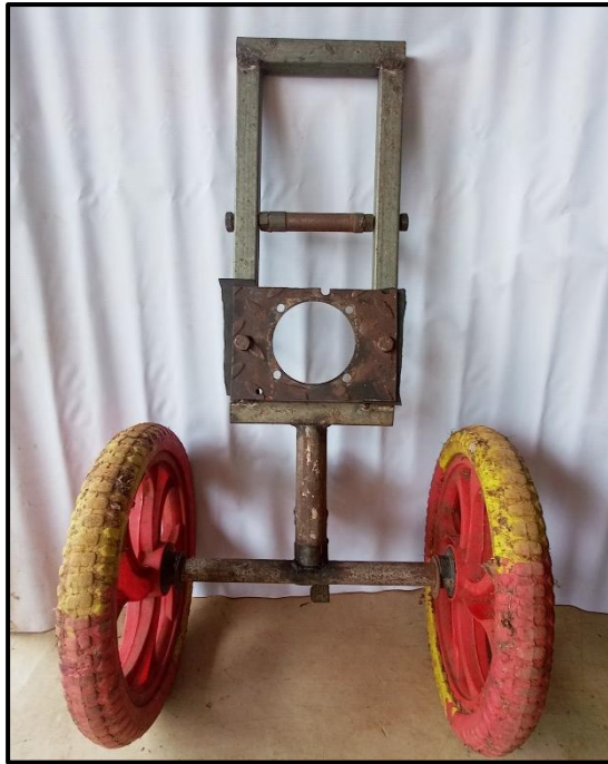
(a) Transport wheels and axel with engine mountning frame
