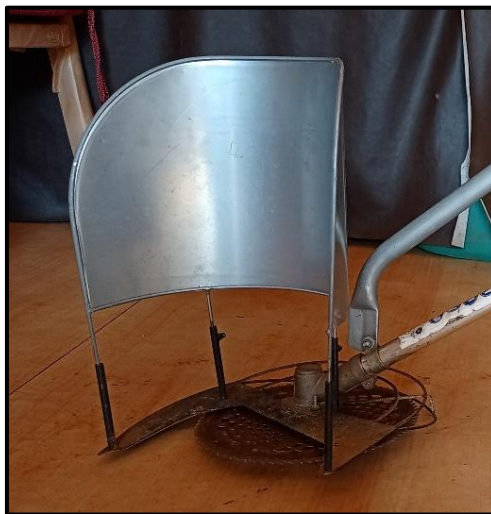
(b) Cutter blade with windrowing attachment
