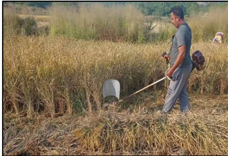
(c) Operation with shoulder mouted brush cutter
