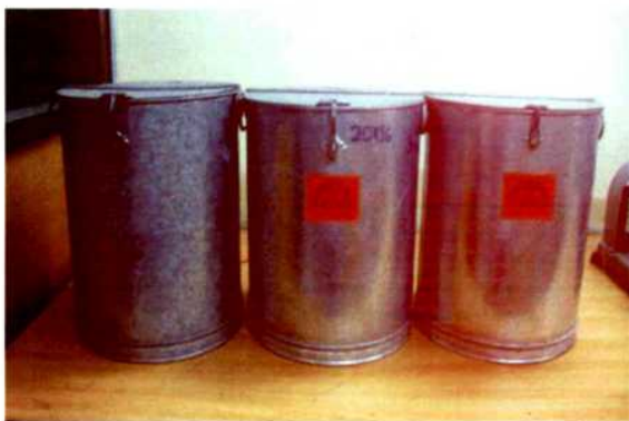
Plate 3.10: Galvanized Iron Bin (GI), [sheet thickness 0.50 mm]
