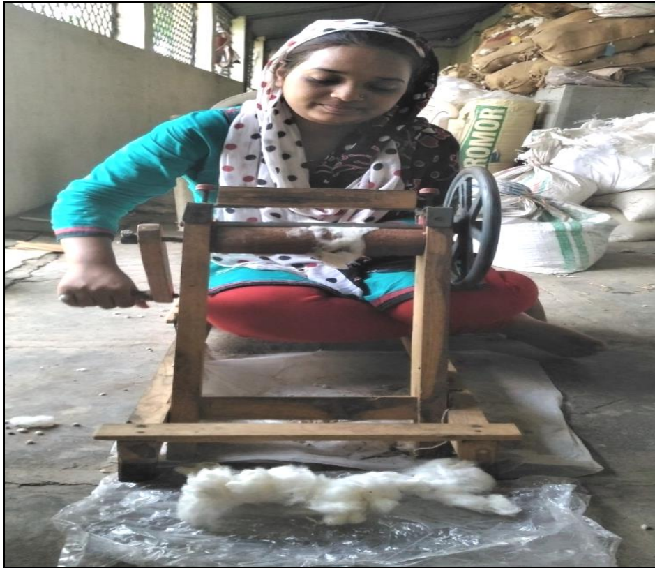
Plate 8. To separate the lint from the seed cotton yield by using ginning hand machine
