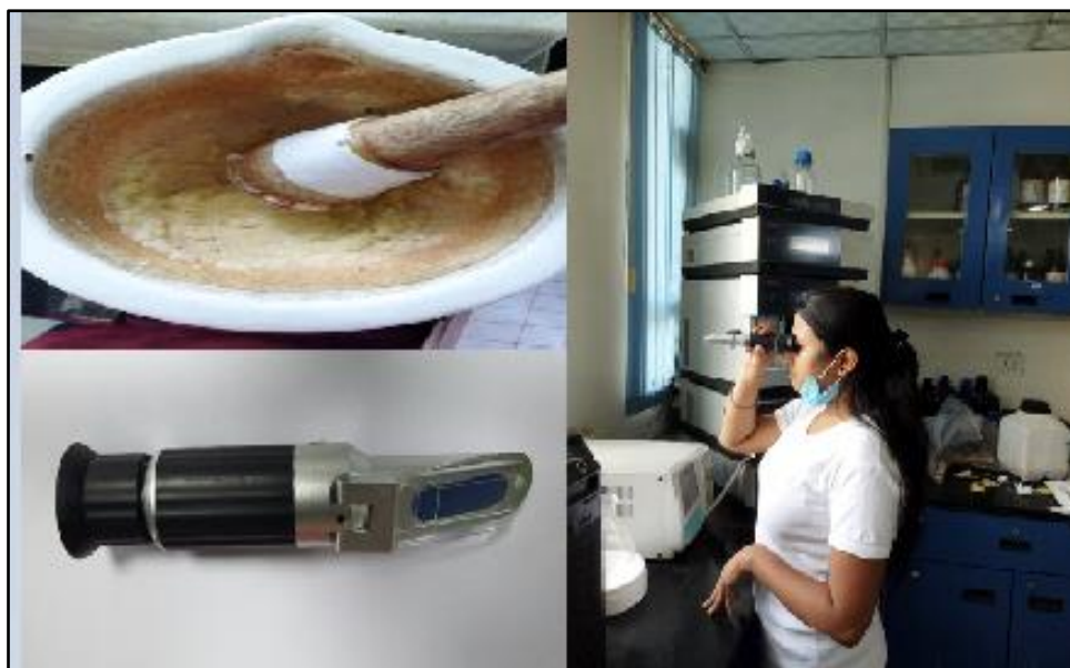
Plate 3.14. Sample preparation and measurement of TSS content by Refractometer
