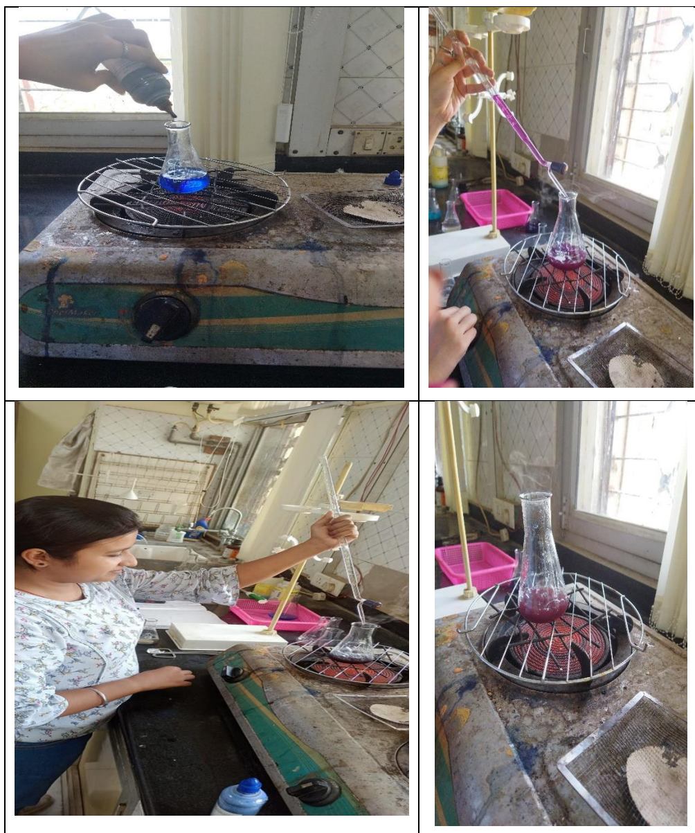
Plate 3.17. Measurement of total sugar and reducing sugar content in gas flame
