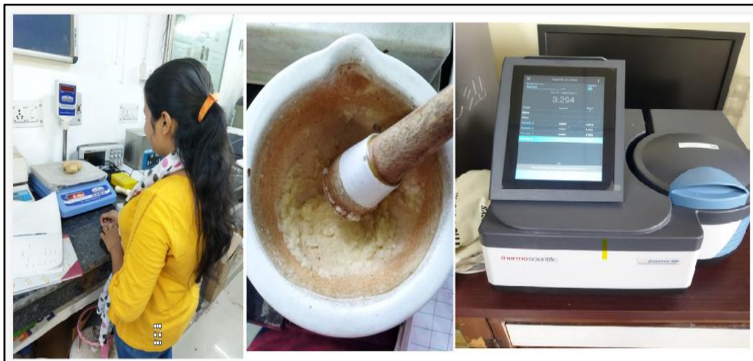
Plate 3.15. Sample preparation and measurement of Starch content by Spectrophotometer
