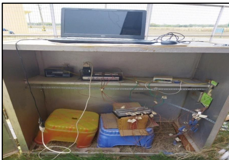
Plate 3.2. Data logger and multiplexer set-up for measuring temperature
