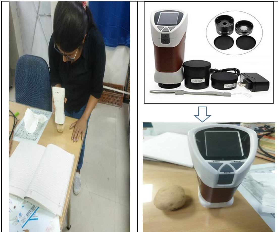
Plate 3.13. Measurement of L*, a*, b* values by colorimeter
