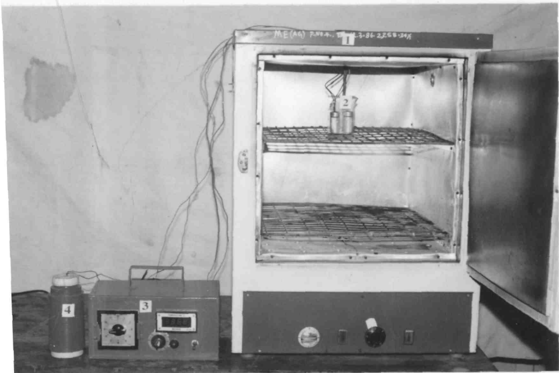
PLATE 3. Experimental set up for measuring specific heat
