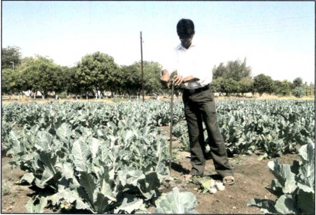
Plate No. 3.3 Taking the soil samples from the experimental plot with screw auger for moisture content determination
