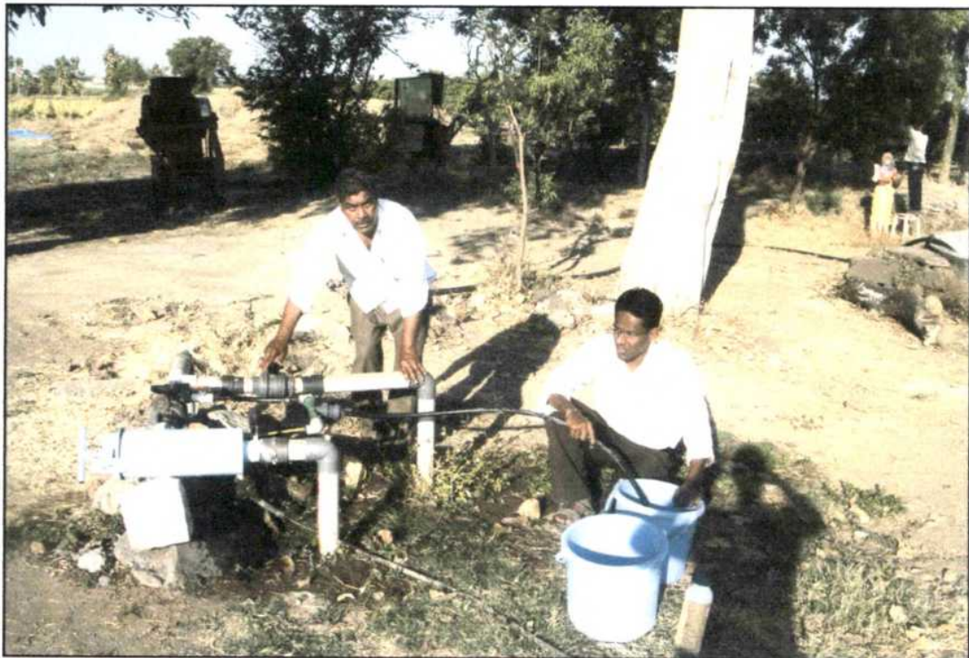
Plate No. 3.2 Fertilizer application through Ventury
