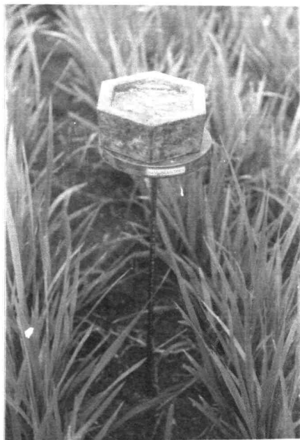
Plate 8: Graduated steel rod with weight used to
