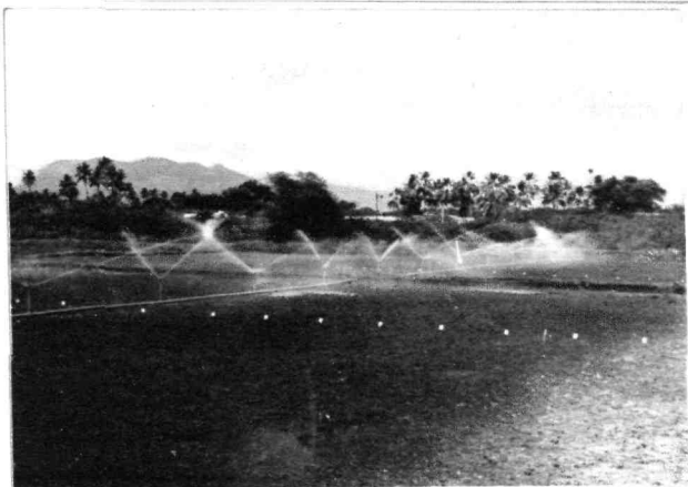
Plate 1. Line source sprinkler system in operation and catch cans placed at right angle to the sprinkler line
