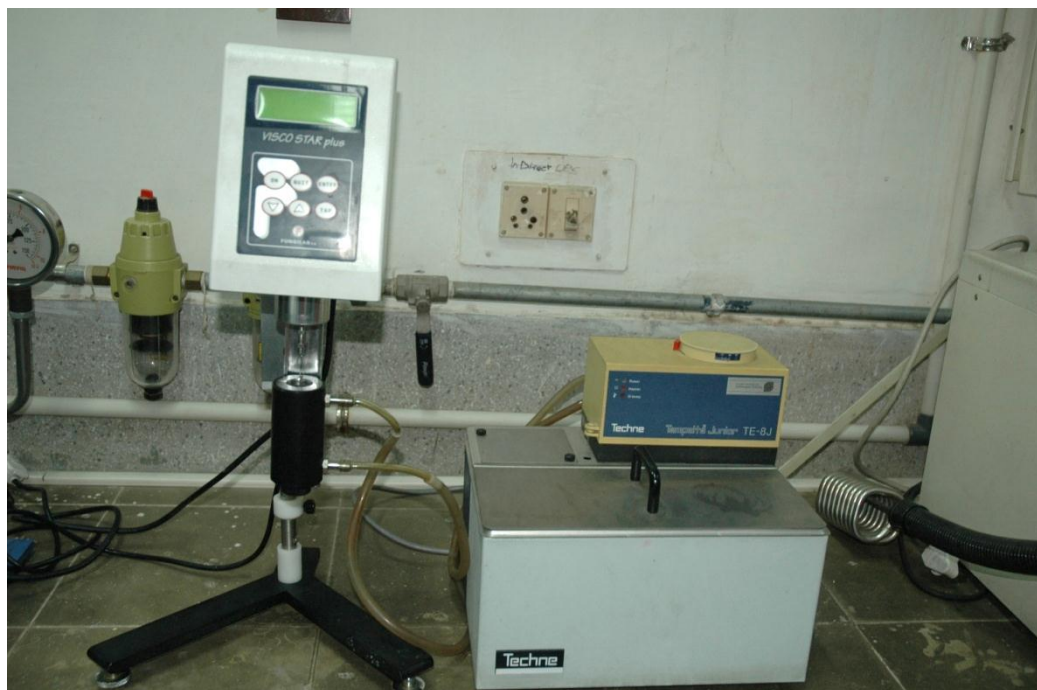
12. Viscometer for viscosity measurement
