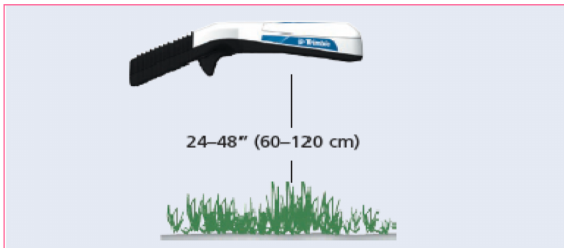
Fig. 5: GreenSeeker hand held optical sensor's position during sensing the crop
