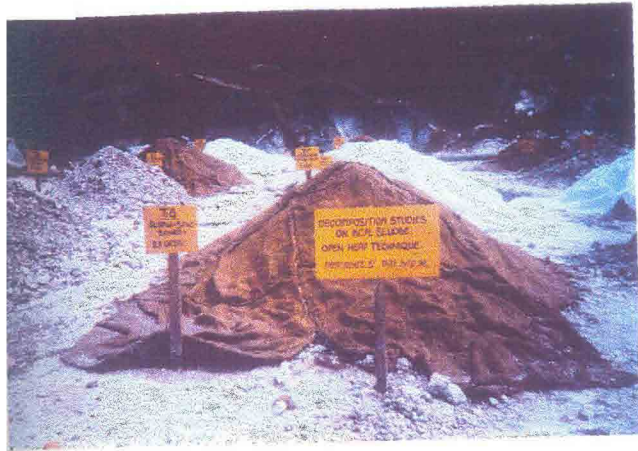
Plate 12 Aerobic open heap composting technique
