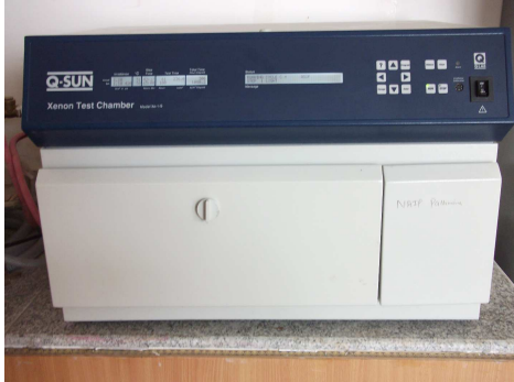
Light fastness by Xenon test chamber (Model Xe-1-S, Q-SUN)
