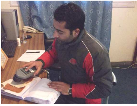
Colour attributes by Chromometer (Model CR-2000, Minolta, Osaka, Japan)
