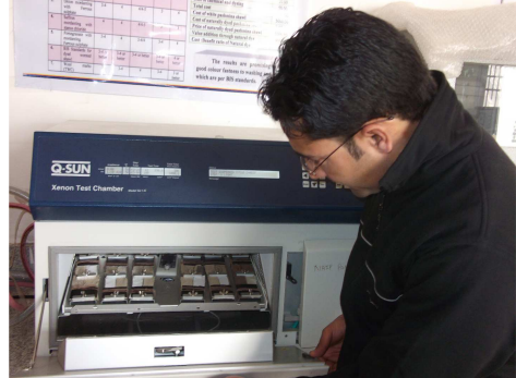
Light fastness by Xenon test chamber (Model Xe-1-S, Q-SUN)
