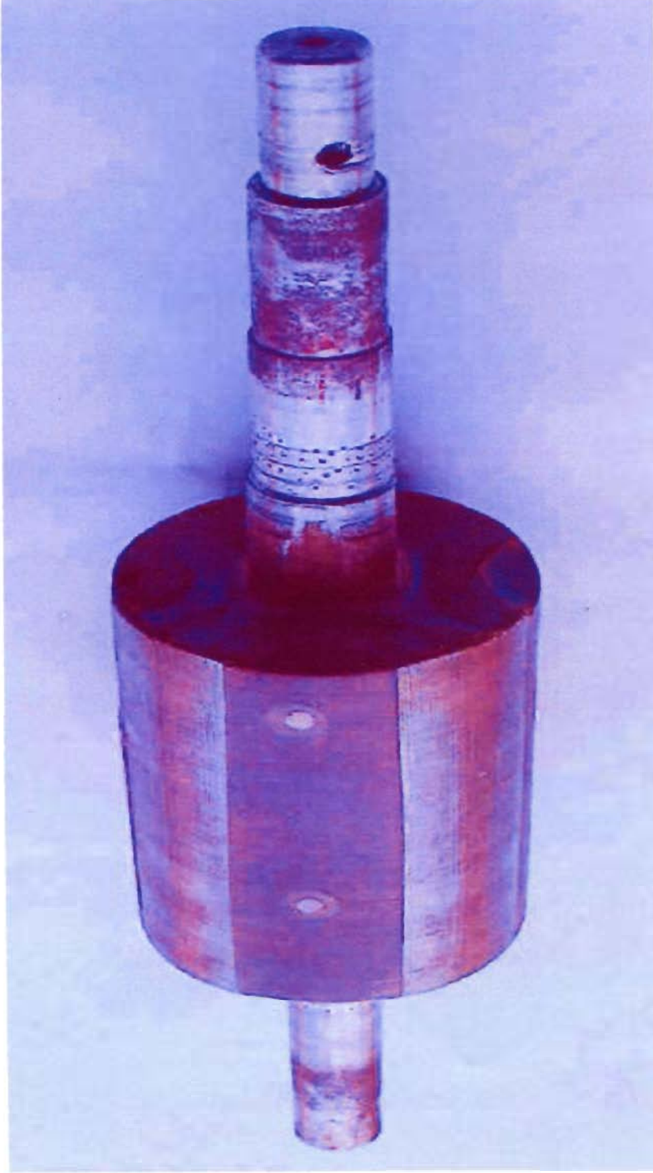
Fig.4.3 Fabricated 4-poles axially laminated anisotropic rotor
