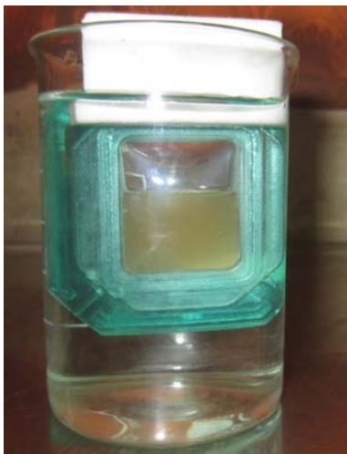
Fig. 1b: Dialysis of silk fibroin with 3500 MWCO Slide Lyzer Cassette with float.
