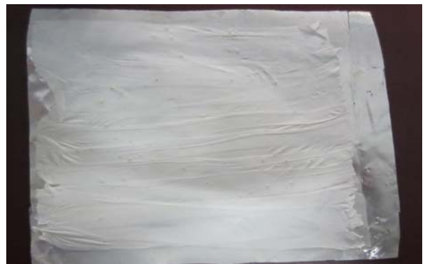
Fig. 1e: Electrospun silk fibroin sheet with 0.5 mm thickness and 2-5 \mu\text{m} porosity.
