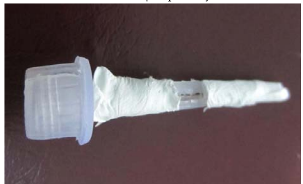
Fig. 1f: Electrospun silk fibroin sheet rolled teat plug for clinical trial.
