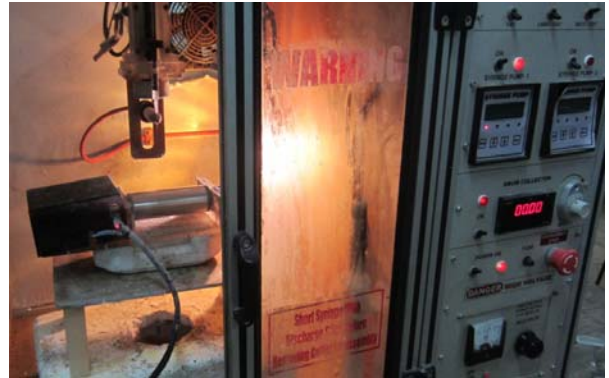
Fig. 1c: Electrospinning of silk fibroin at IIT Chennai.
