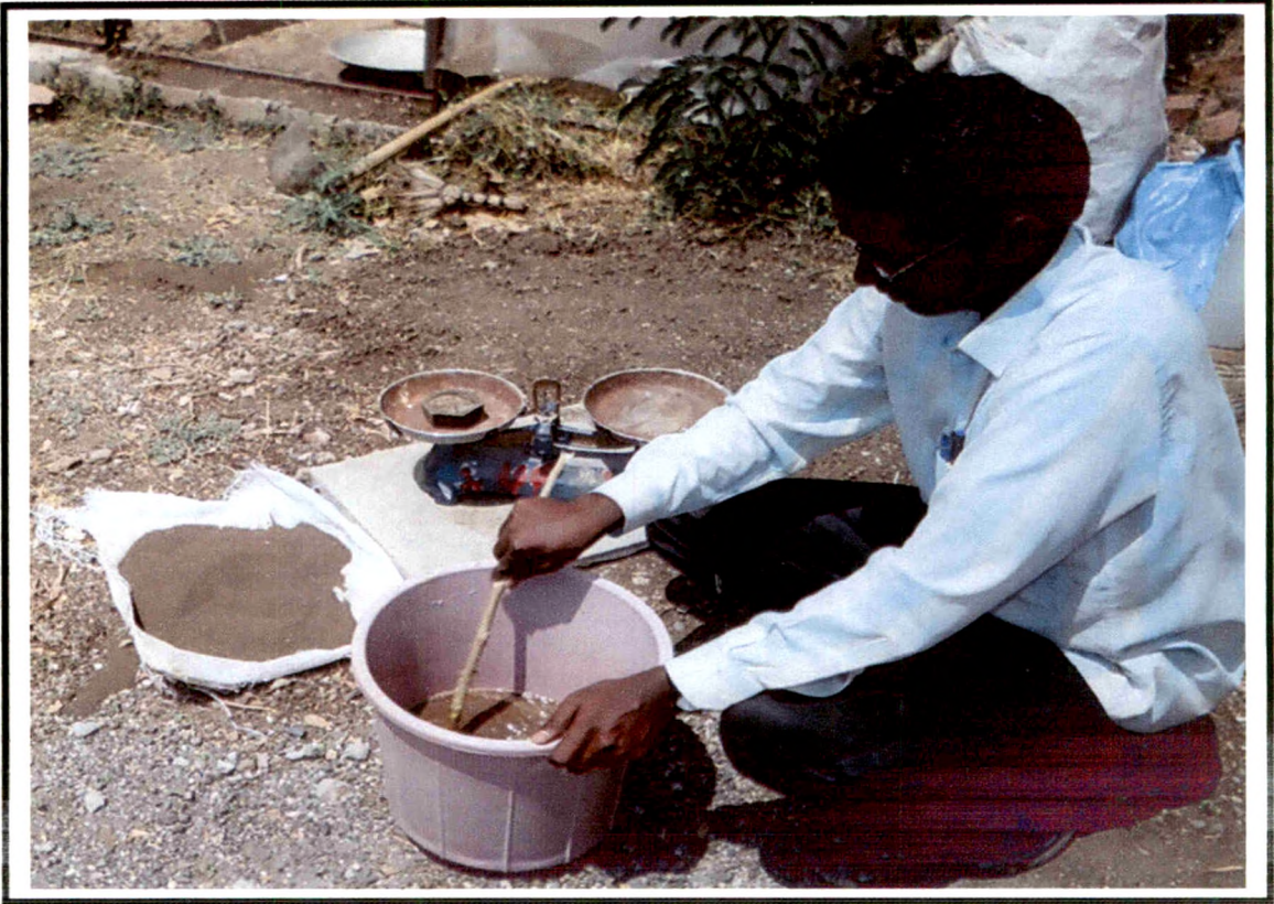
Plate 8 : Preparation of soil paste
