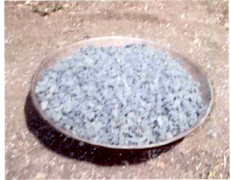
Angular gravel grade II
