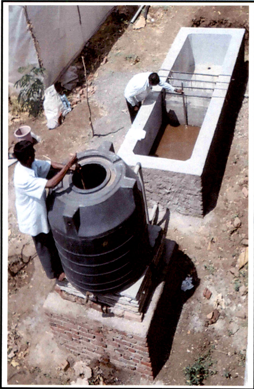
Plate 6 : Measurement of inlet head
