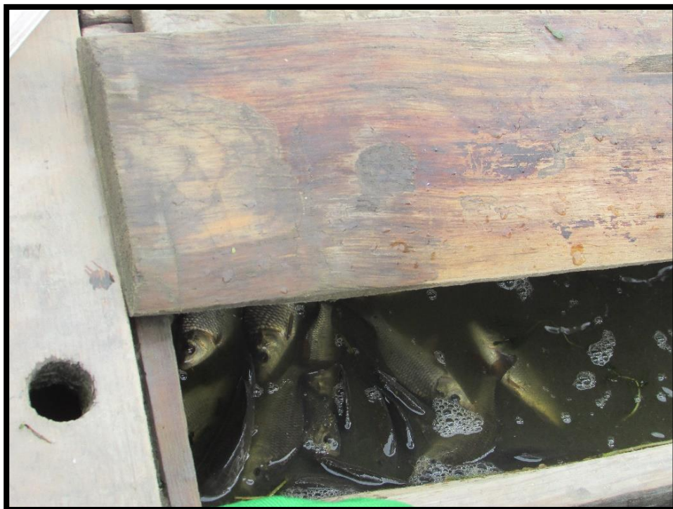
Plate 4: Fish hold provision in few boats, redesigned fishing craft
