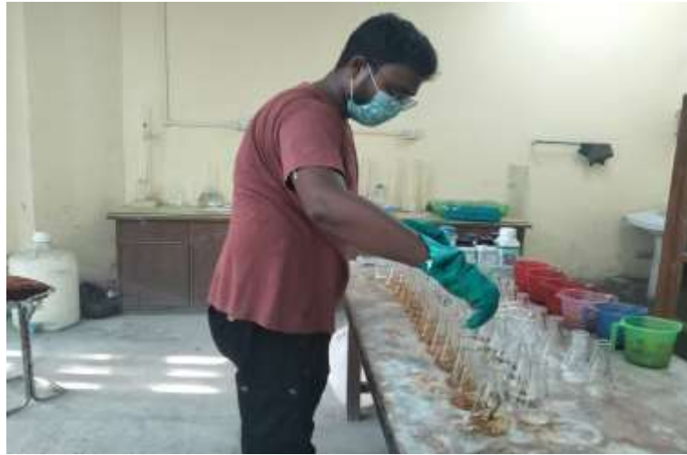
Plate No. 1: Addition of Tri acid mixtures in plant samples
