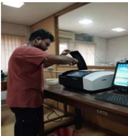
Plate No. 5: Phosphorus analysis of soil samples using spectrophotometer
