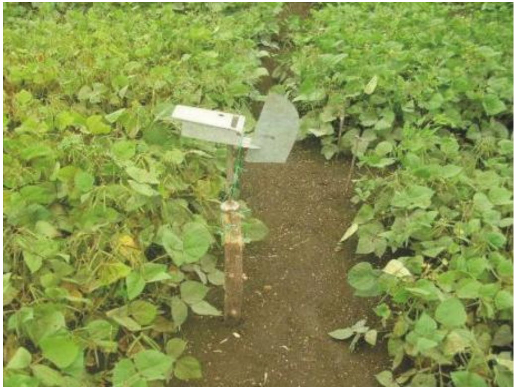
Plate 11b. Spore trap mounted in greengram experimental field for sampling of air borne conidia
