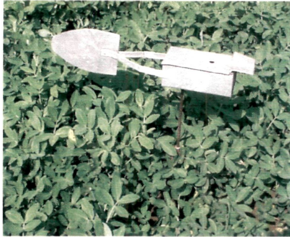
Plate 8a. Trapping of uredospores by mounting aeroscope in the groundnut field.
