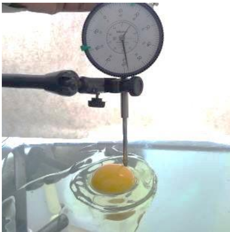
Plate 3.6 Estimation of albumen height using dial test indicator
