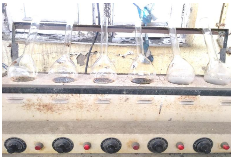
Plate 3.3 Digestion of samples for Crude protein estimation
