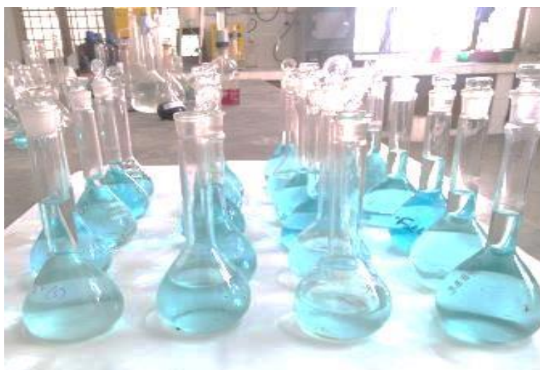
Plate 3.4 Digested samples in volumetric flasks for estimation of Crude protein
