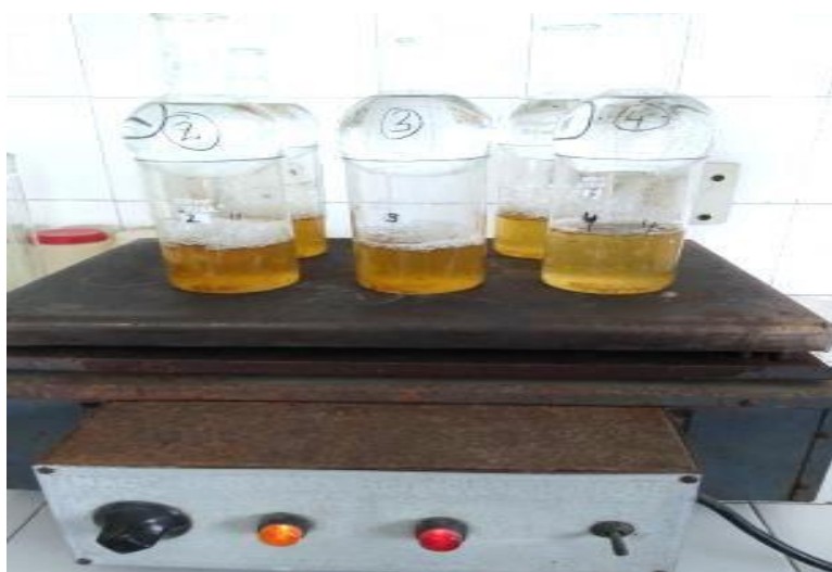
Plate 3.5 Crude fibre estimation of samples by treatment with acid and alkali
