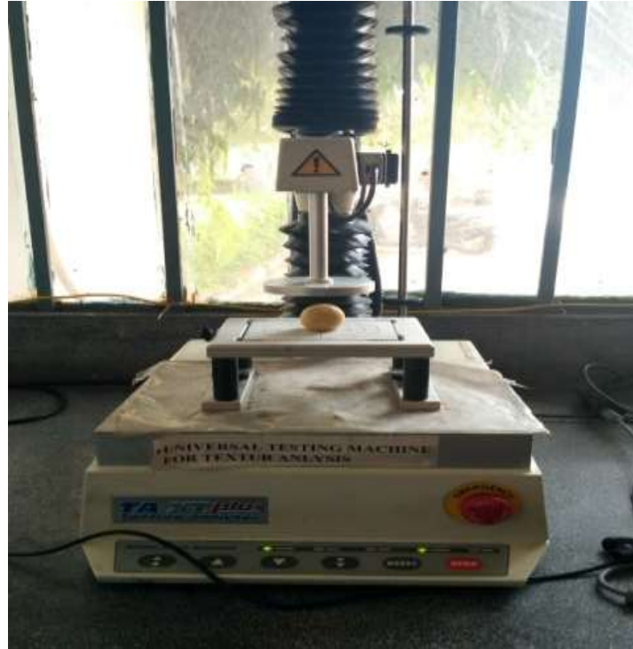
Fig. 3.7 Universal testing machine for texture analysis
