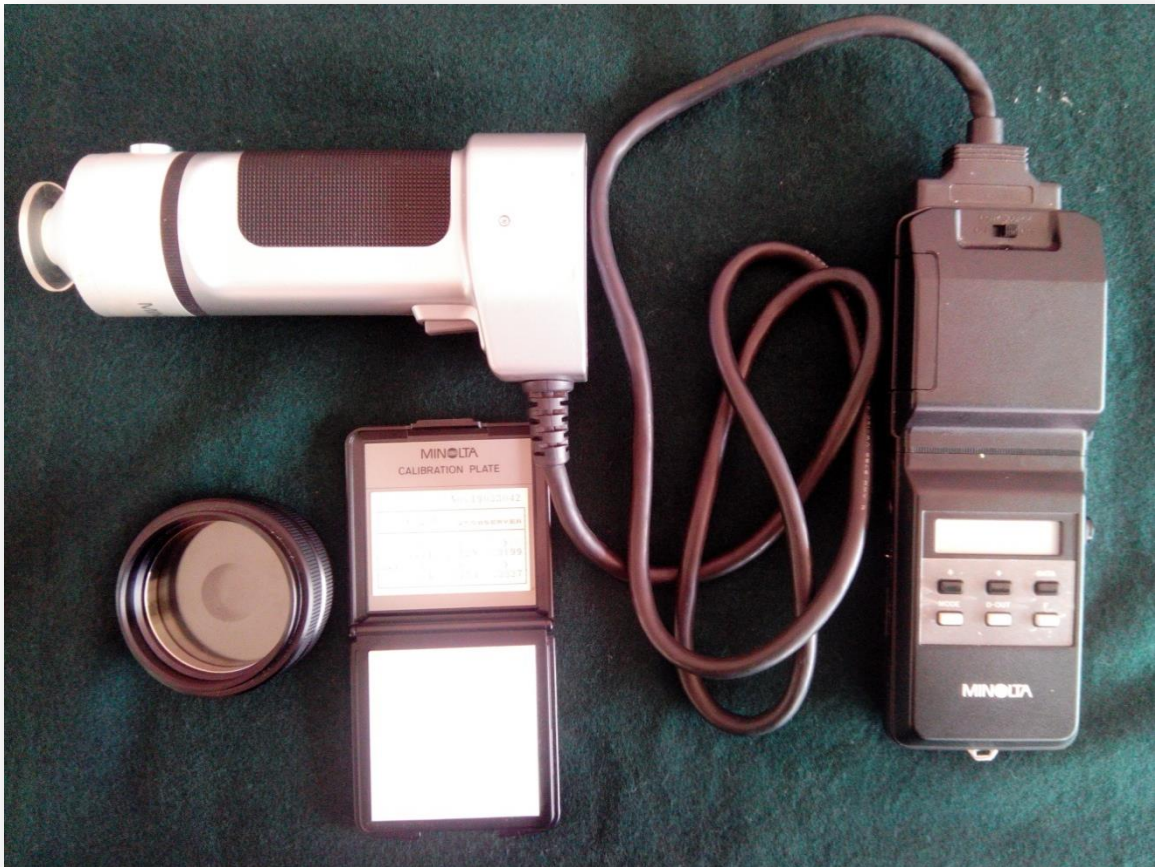
Plate 1: COLOURIMETER CR-200b (Minolta Chroma Instrument, Japan) used for the assessment of colour
