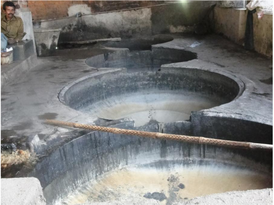
Plate 1: Four Pan system for efficient jaggery making
