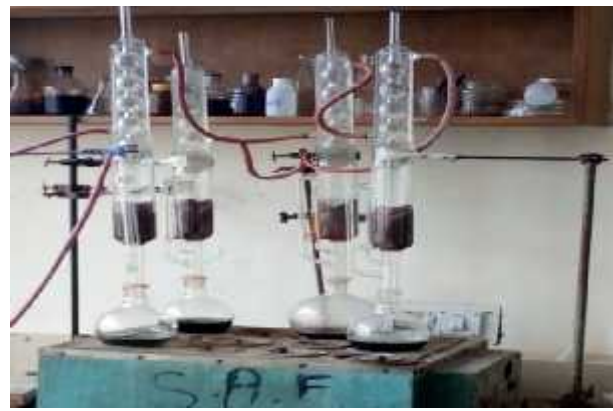
c. Alcohol: benzene extraction using Soxhlet
