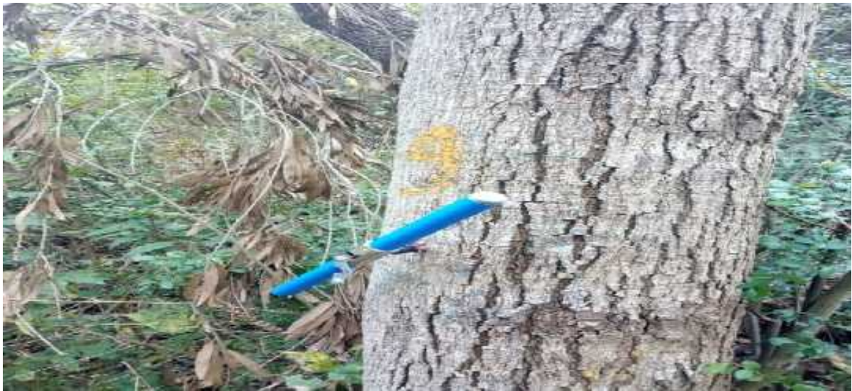
a. Extracted sample using Increment borer
