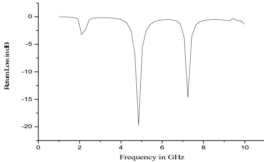
Figure: 4.7: Return loss Vs frequency plot of pentagonal shape antenna
