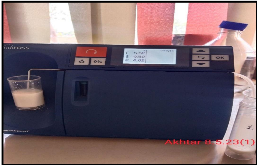
Plate 3.7: Estimation of Fat%, Protein% and SNF% in milk samples using milk adulteration scanner & quality analyser (Milkoscreen™, Indifoss Analytical Pvt Ltd., USA)
