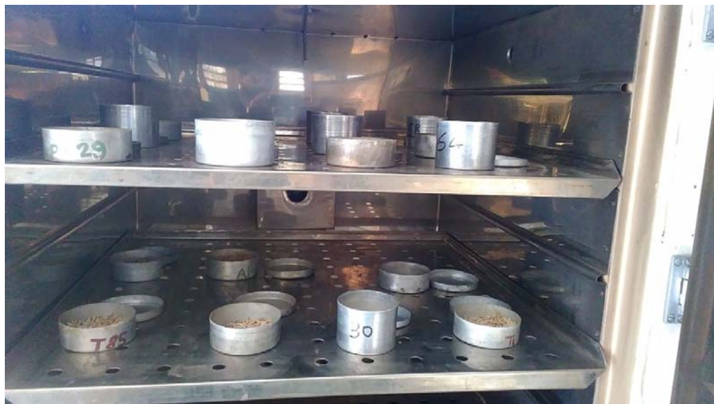
Plate 3.1: Hot air oven for determination of moisture content
