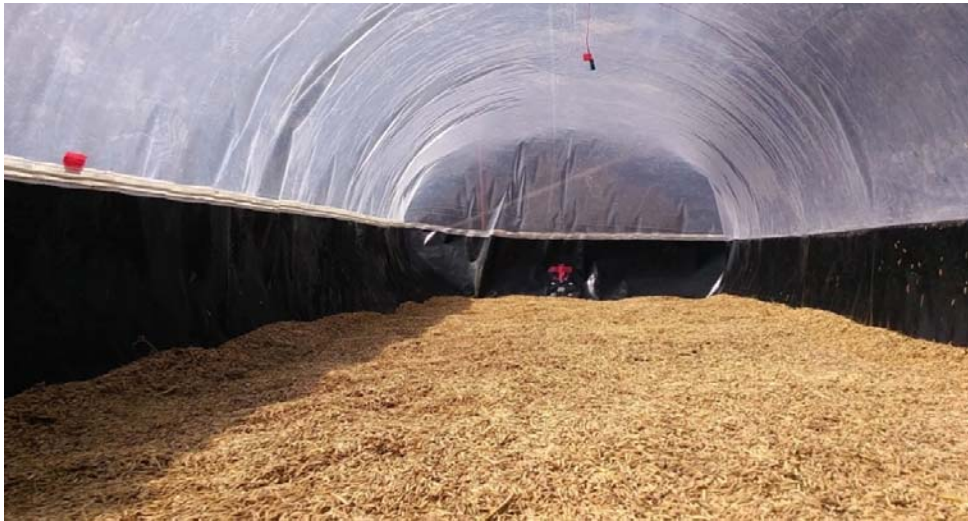
Plate 3.5: Grain bed in the drying chamber
