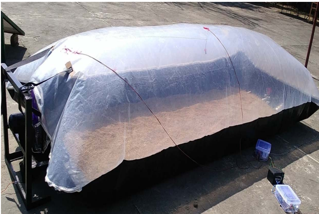
Plate 3.3: Fabricated drying chamber of solar powered air inflated grain dryer
