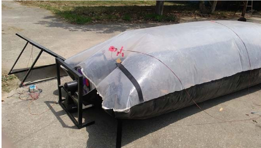
Plate 3.4: Developed solar powered air inflated grain dryer
