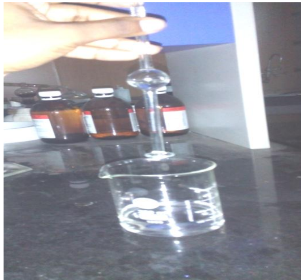
Fig. 3.11 Measurement of surface tension of Cassia tora seed gum
