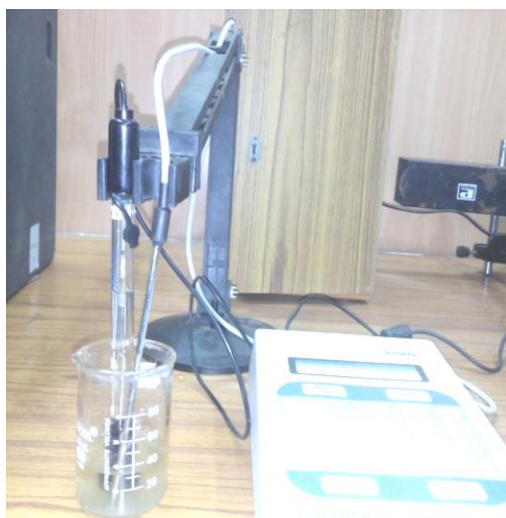
Fig. 3.10 pH measurement of Cassia tora seed gum
