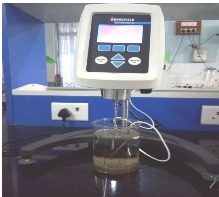
Fig. 3.12 Measurement of viscosity of Cassia tora seed gum
