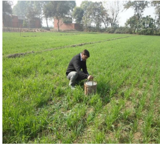
Fig. 3.9b. Infiltration measurements in wheat field
