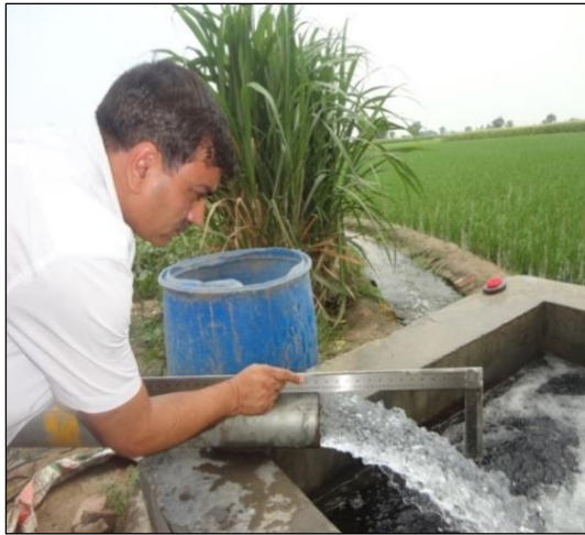
Fig. 3.3a. L - shaped gauge for discharge measurement
