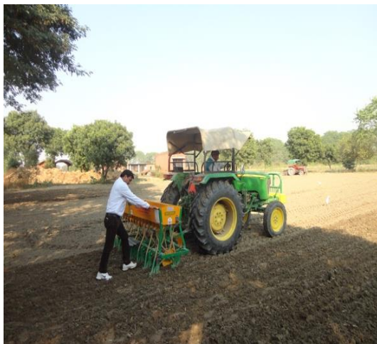
Fig. 3.7e. Wheat sowing by seed cum fertilizer drill
