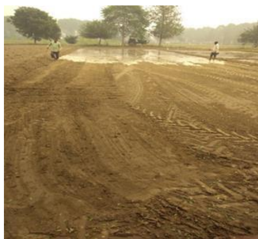
Fig. 3.9d. Water advance measurement in laser levelled field
