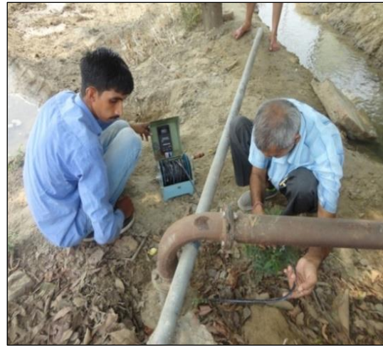
Fig. 3.3b. Electronic water level indicator
