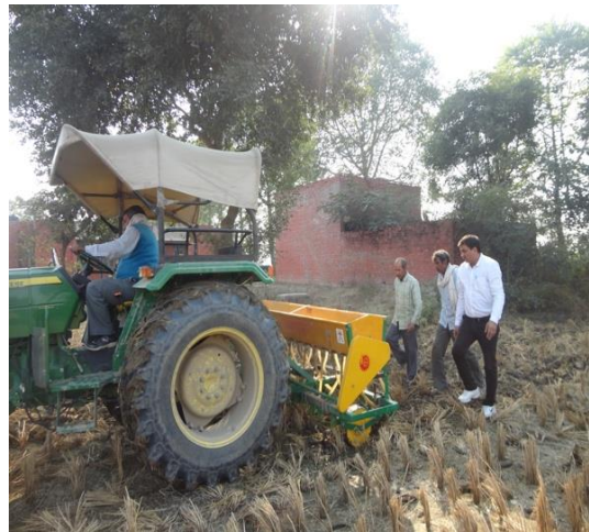
Fig. 3.7d. Wheat sowing by zero tillage
