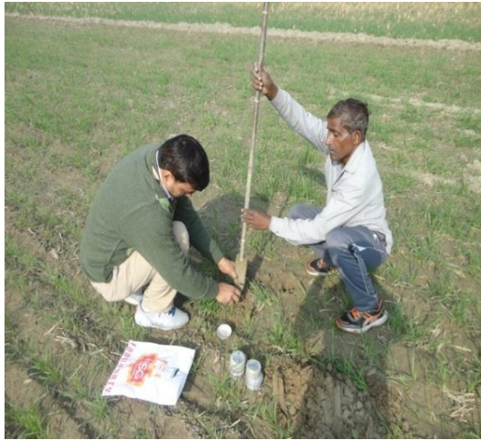
Fig. 3.9a. Soil sampling for moisture content
