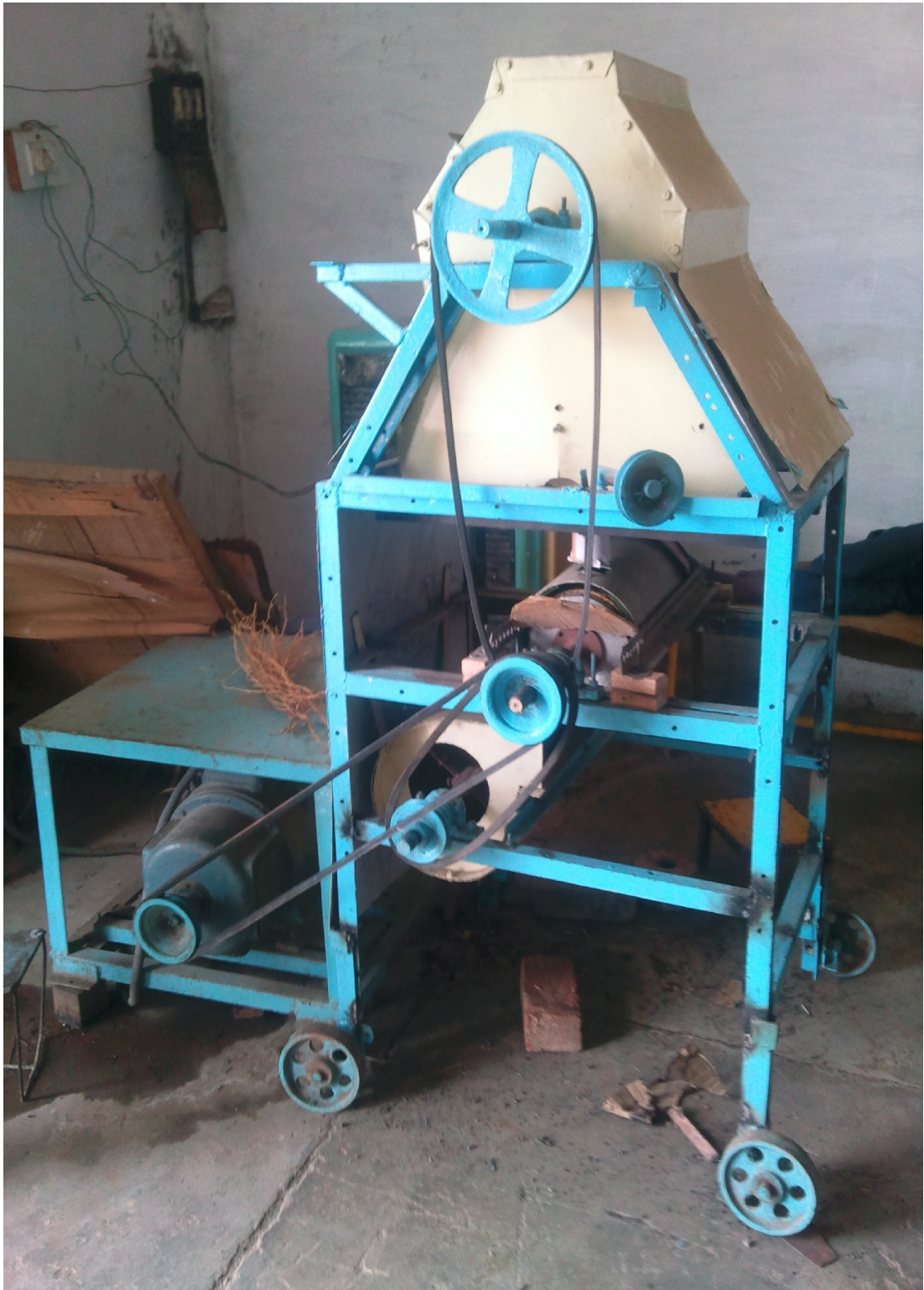
Plate 4.1 Modified Green Chickpea Pod Stripping cum Shelling Machine.
