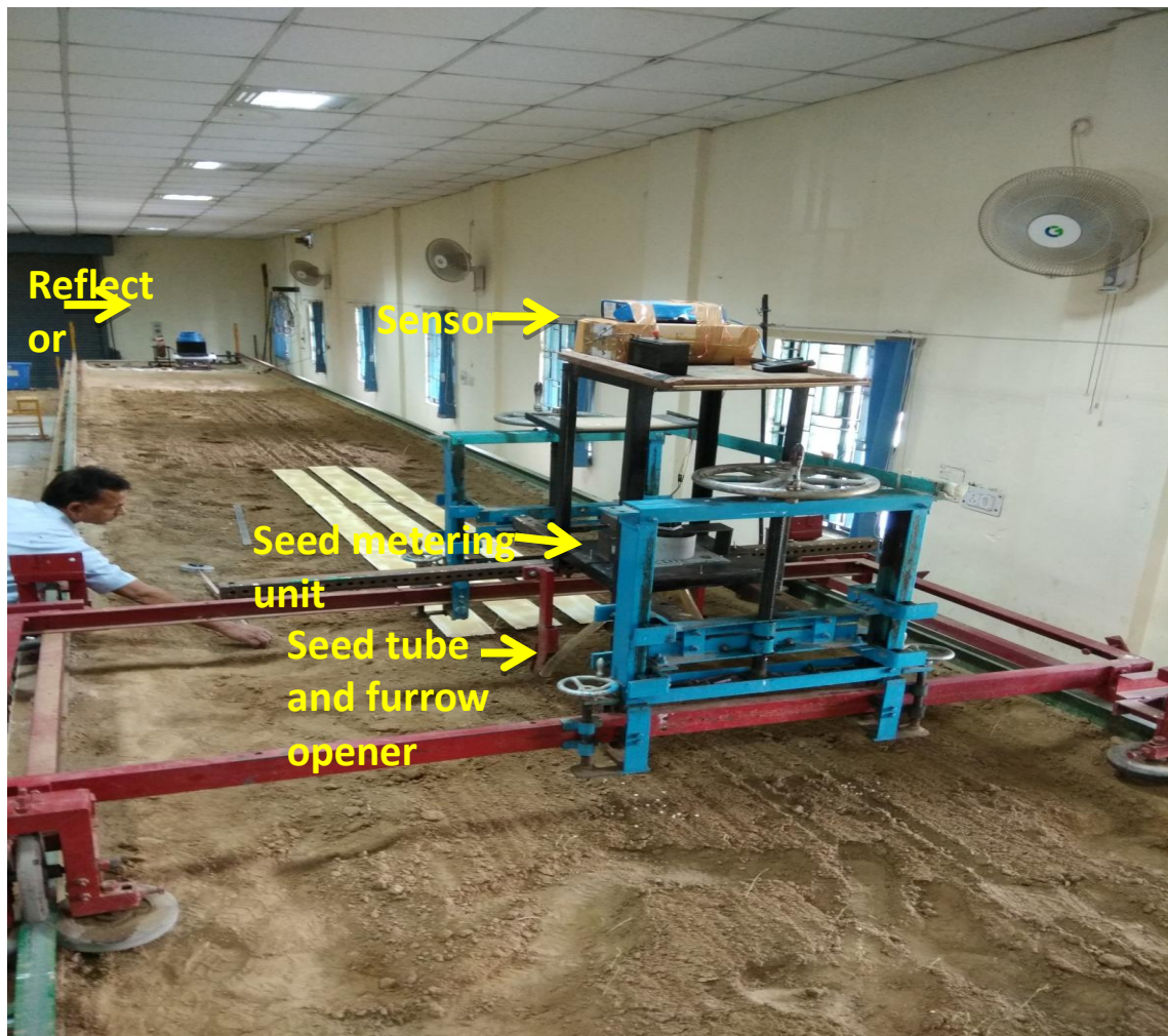
Plate 3.10 Sensor controlled check row plating system mounted on soil bin platform
