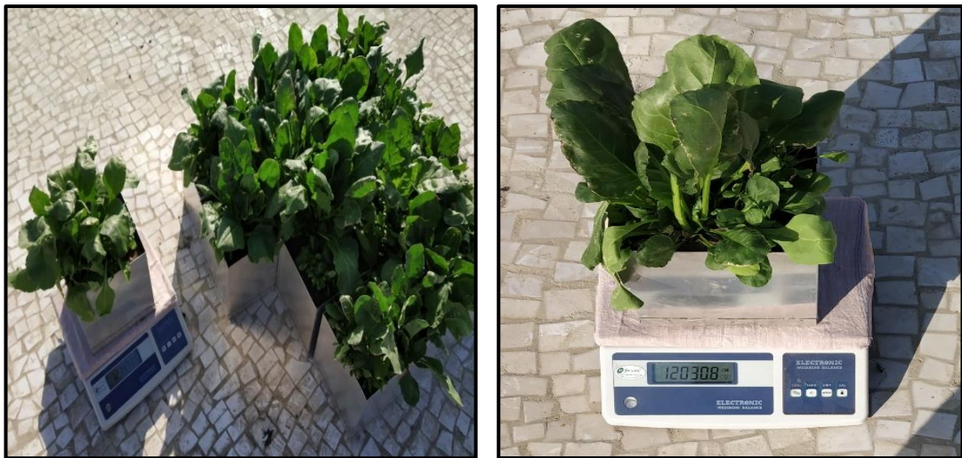
Plate 3.6 ET c measurements by micro-lysimeters
