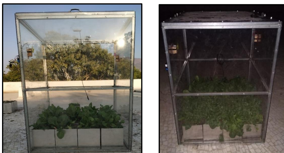
Plate 3.4 Measurement of evapotranspiration in the closed canopy chamber
